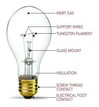
Electricity flows through a thin tungsten wire (FILAMENT) in the Incandescent light bulb. The filament used in this bulb has a property called "resistance". A filament has a lot of resistance to electricity. As a result of this resistance, the filament heats up and start glowing, converting electrical energy to light energy.
